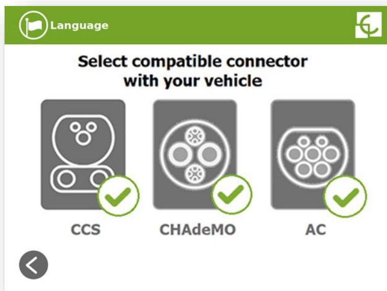
**The connector can be removed from the holder by selecting it on the station screen:**
